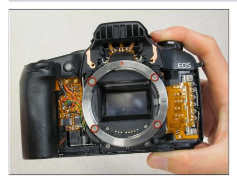
• Remove four 7.1 mm silver screws from lens mount ring.
