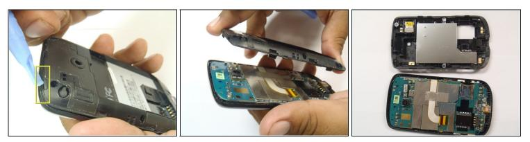
• Pry the frame open, releasing the eight plastic tabs around the edge of the frame, using the plastic opening tool.
