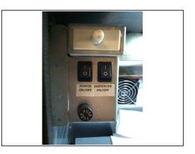
• The UPC is located at the bottom right of the machine. Before removing it you should shut down the kiosk and power down the machine via the two switches on the top left of the machine.
