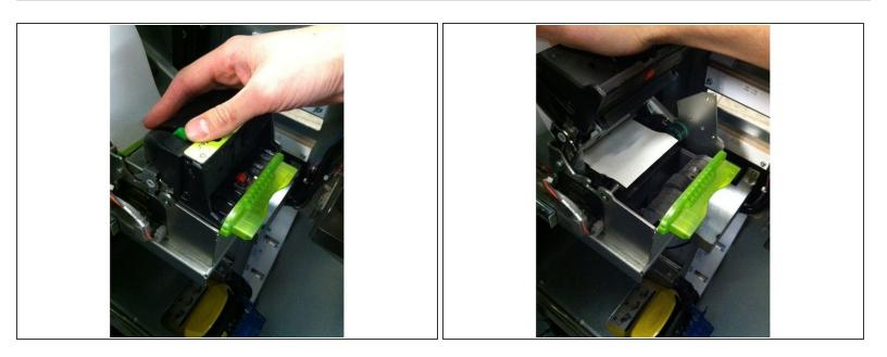
• Open and blow out the printer to remove any loose paper
