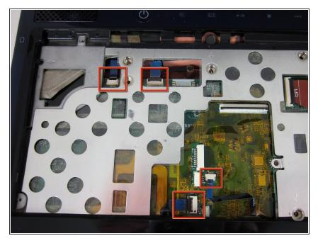
Detach the four blue ribbon cables carefully with tweezers. Some of the ribbons may require a flap to be raised because it secures the ribbon in.
