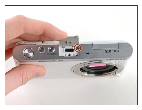
Remove the 4 mm Phillips #00 screw hiding in the external flash port.
