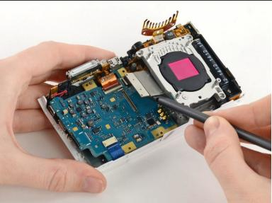
Use a spudger to disconnect the ribbon cable connecting the image sensor to the motherboard.
