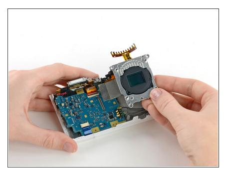
Gently remove the sensor mount from the camera case.
