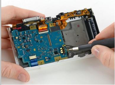
• Use a Phillips #00 screwdriver to remove the 3 mm screw located below the wifi antenna.
