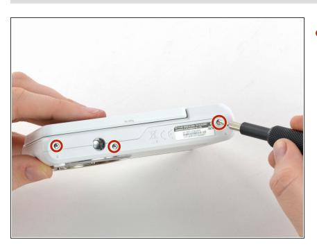
Use a Phillips #00 screwdriver to remove the three 4 mm screws from the bottom of the case.
