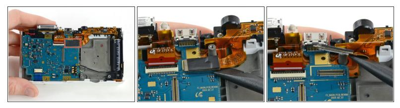
• Use a spudger to disconnect the LCD ribbon cable by prying it straight up from the motherboard.
