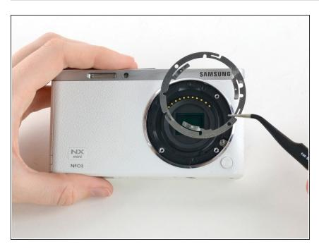
Use tweezers to remove the inner metal ring.
