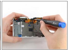
• Use a Phillips #00 screwdriver to remove the two 5 mm screws holding the flash assembly to the camera case.
