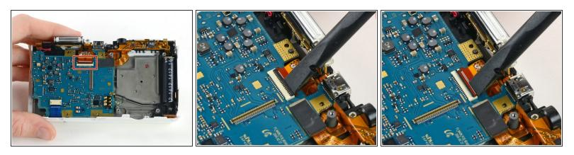
Use a spudger to unlock the topmost ZIF connector by flipping open the black flap.
