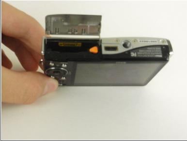
Slide the battery door in the direction of the arrow, toward the LCD screen. The door will then swing open.
