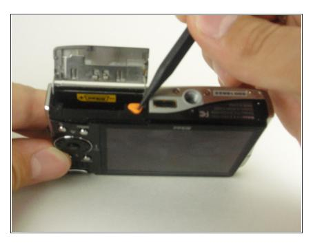
Push the orange release mechanism with the spudger in the direction of the arrow, freeing the battery.
