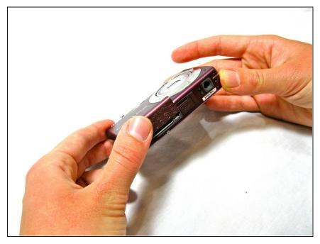
Slide the battery and memory card cover (located on the bottom of the camera) to release it.
