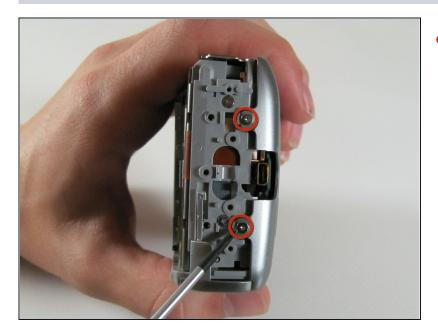
Remove the two 4.6 mm screws attaching the front panel to the body on the left side.
