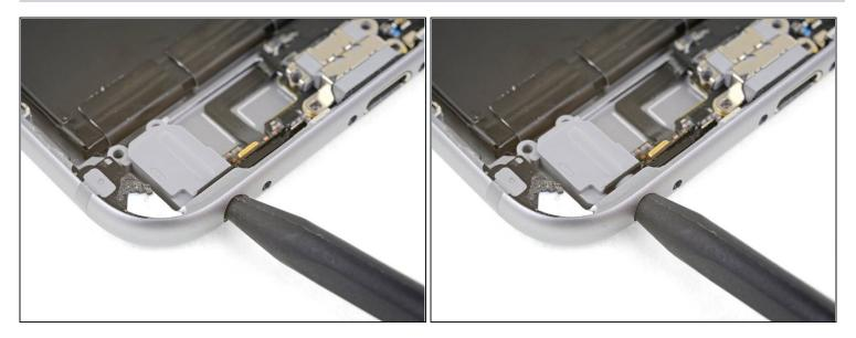
• Insert the point of a spudger into the headphone jack and wiggle it slightly to loosen the headphone jack from the bottom edge of the case.
