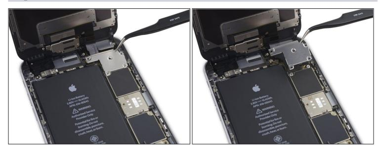
• Remove the display cable bracket.
