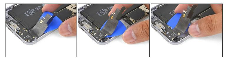
• Continue sliding the opening pick underneath the flex cable.
