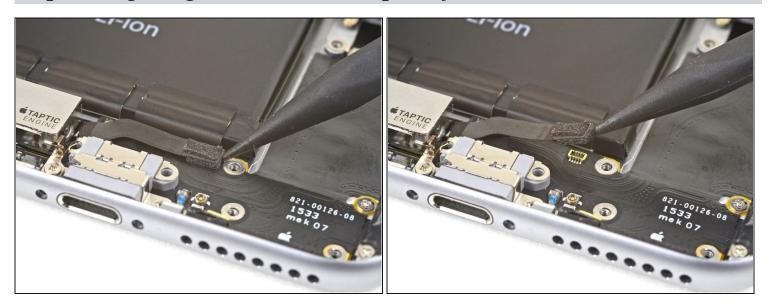
• Use the point of a spudger to disconnect the Taptic Engine flex cable from the lower flex cable.
