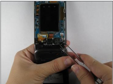
• Use tweezers to insert the new speaker into the speaker slot.
