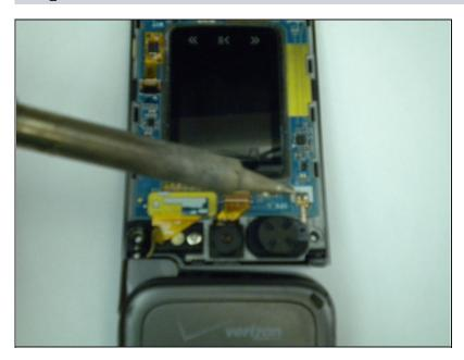
Use soldering iron to melt, and remove soldering joints of the speaker.
