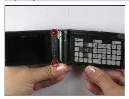
• Remove the two (4.1 mm) screws down the screen.
