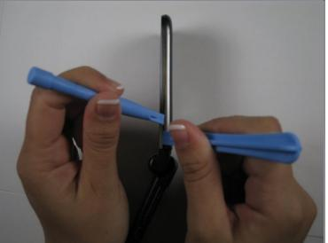
Remove the upper casing with a plastic opening tools.
