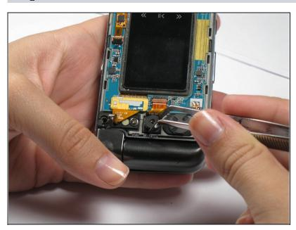
Use <u>tweezers</u> to remove the camera from its holding slot.
