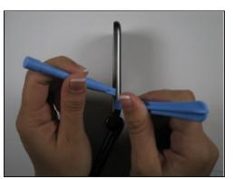
Remove front outside casing with plastic opening tools.
