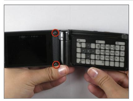
• Remove the (2) 4.1 mm screws on screen.
