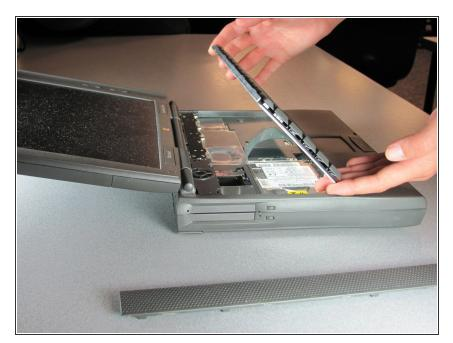
Gently lift the keyboard until only the ribbon cable remains attached.
