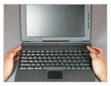
Press firmly on each end of the speaker cover and slide it to the left.
