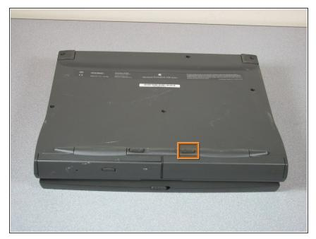
Turn the device upside down and then locate the battery latch near the front of the device.
