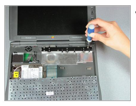
Remove the six screws from the heatsink using the Philips #1 screwdriver.
