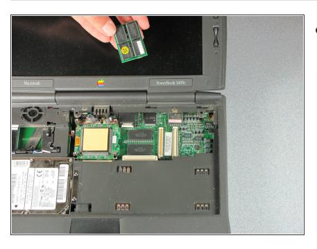
Remove the factory installed RAM memory module
