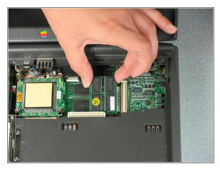
Gently grasp the factory installed RAM by grabbing each end as shown in the picture and pull the stick directly up
