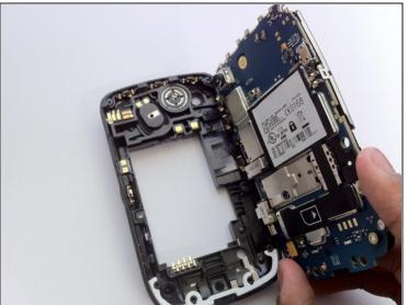
• Using a plastic opening tool, gently pry the motherboard assembly from the device's frame.
