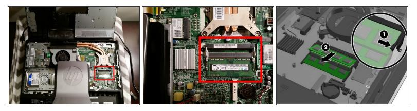
• Locate the SODIMM slots. To remove the memory module, press outward on the two latches on each side of the SODIMM, then pull the SODIMM out of the socket.
