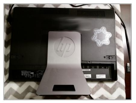
Place the computer face down on a soft, flat surface. A blanket, towel, or other soft cloth will protect the bezel and screen from scratches or other damage.
