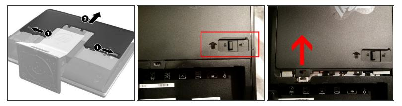
• To remove the cover: slide the latches on the right and left sides of the back cover towards the edges of the unit, then slide the cover towards the top of the computer until it slides off the unit.
