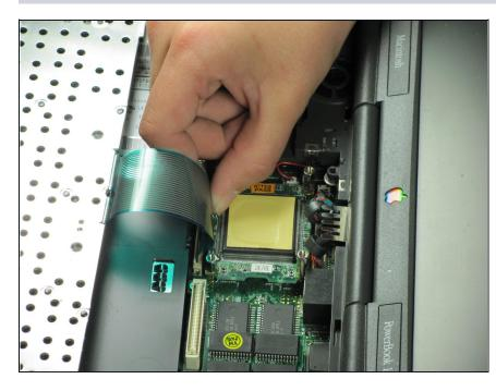
• Gently pull up on the beige ribbon lock until it moves a short distance on both sides to separate the ribbon cable from the connector.
