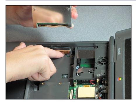
Remove the hard drive from the computer by pushing down on the plastic strap and pulling up on the hard drive.
