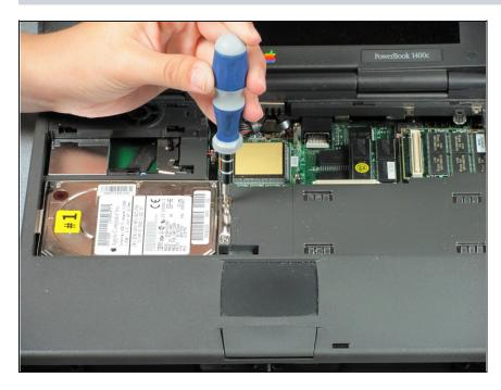
Remove the screws with a Phillips #0 screwdriver.
