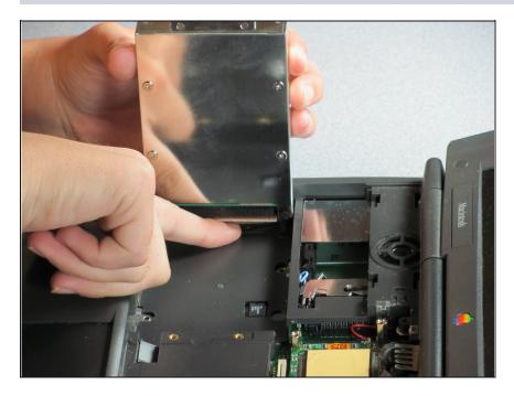
• Push a finger down onto the plastic strap.
