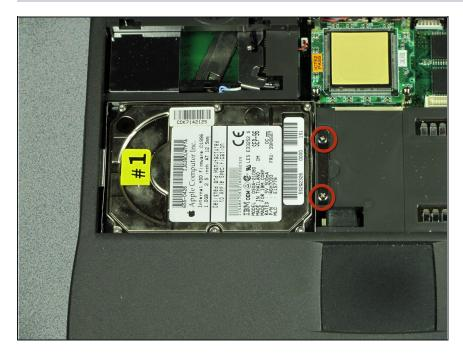
• Locate and identify the two screws that attach the hard drive to the computer.
