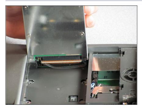
• Fully lift the hard drive vertically against the side of the computer.
