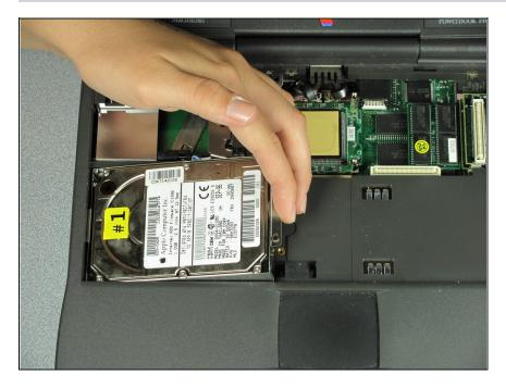
Once the screws are removed, lift up the end of the hard drive using your finger tips.
