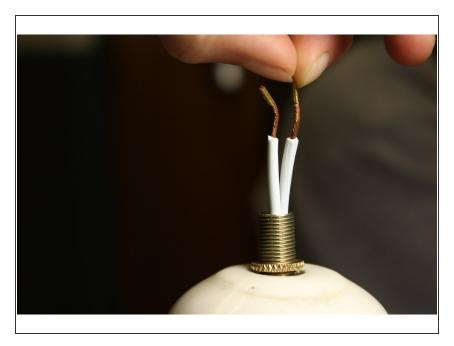
Pull either ends of the wire so that you have about 2-3 inches of the wire separated.
