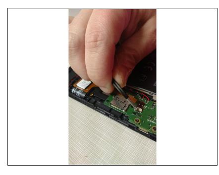
Using your fingernail or tweezers lift the holding flap and disconnect the digitizer cable for the old screen
