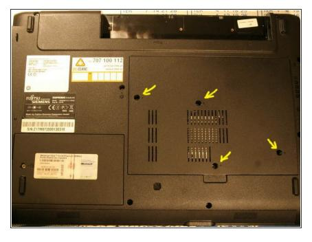
Remove the 4 philips screws that secure the back cover.
