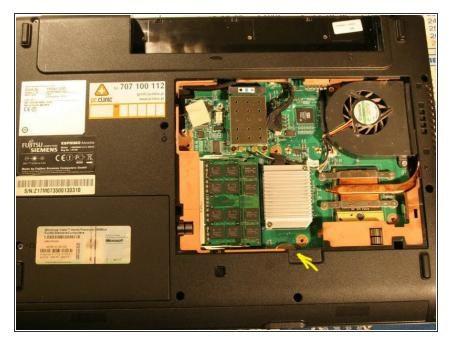
With the cover removed, we can see the battery.
