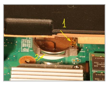
Turn the laptop around so you can see and access the battery. Release the battery with the flat screwdriver (1), then gently push it upward (2). Be careful not to let it slip into the laptop case or you will have to disassemble it completely.
