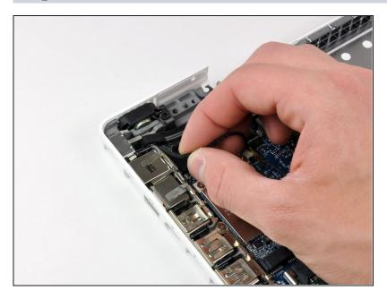
• De-route the left speaker cable from the two clips on the left I/O frame.
