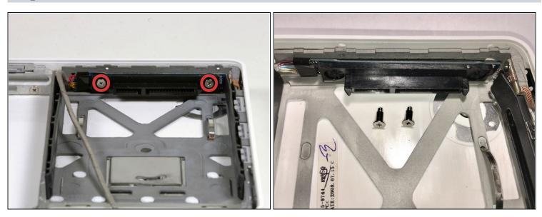
• Remove the two 6 mm Phillips shoulder screws securing the hard drive connector to the lower case.
