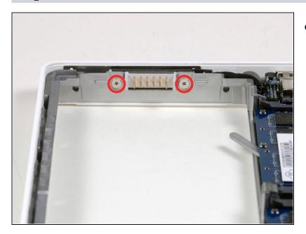
• Remove the two 4 mm Phillips shoulder screws attaching the battery connector to the lower case.
