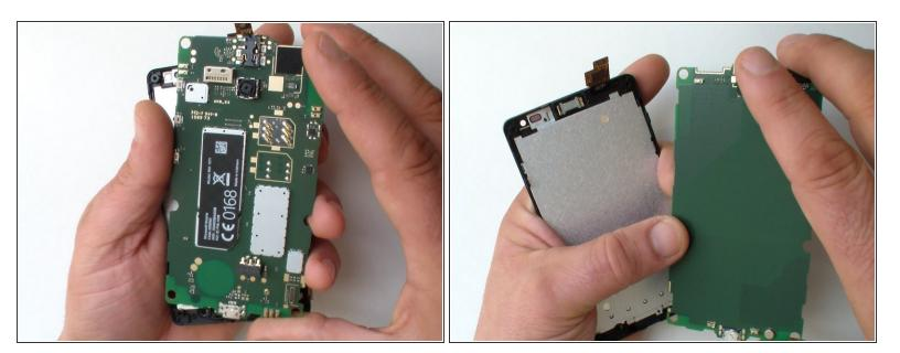
• This is the logic board / main board - a front and rear view.
