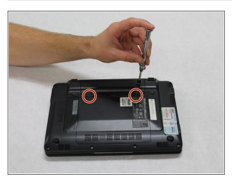
Use a #00 Phillips Head screw driver to remove the two 1/4" screws that hold the back panel in place.
