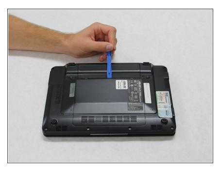
Place the blue plastic 1/4" opening tool into the small indention and gently pry the back panel off.
