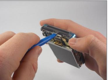
• With a plastic opening tool, gently remove the chrome framing on the left and right sides of the camera.
