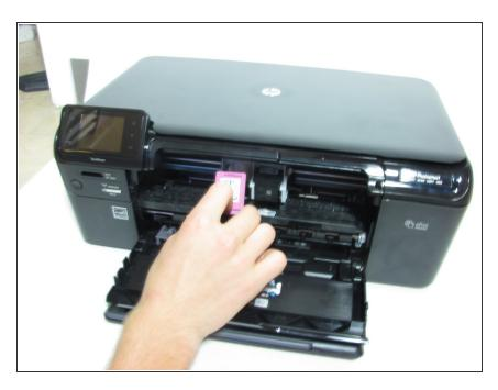
Place the new cartridge into the slot and press firmly until it pops into place.
