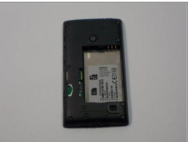
Insert the spudger into the space between the batter and the battery holder to remove the battery.
