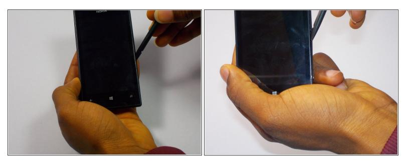
Insert the spudger into the crevice located between the back cover of the phone and the body of the phone.
