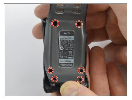
First, place the watch upside down so the back of the watch is exposed. Unscrew the six size #000 5 mm long screws located on the back panel using a size 000 Phillips head screwdriver.
