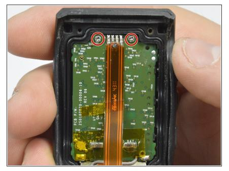
Then, unscrew the two main board size #000 2.5 mm long screws using a size 000 Phillips head screwdriver.
