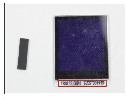
• For reassembly, make sure the highlighted area in the picture, goes over the black plastic piece that was removed in the previous step.
