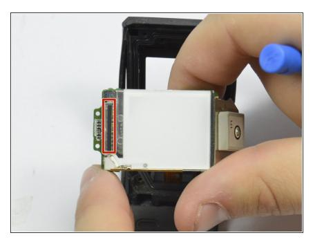
Pull the plastic piece that is highlighted in the picture out from the back of the screen.
