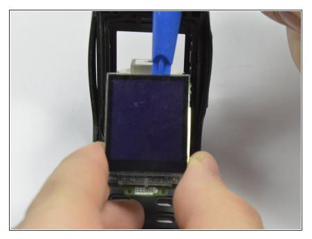
Use the blue plastic removal tool once again to carefully remove the screen.
