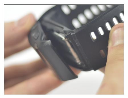
Carefully separate the watch by pulling the band away from the main board.
