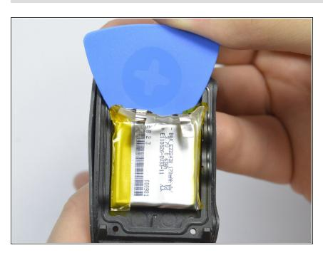
Using a guitar pick removal tool, push under the battery to pry the battery out of the watch.
