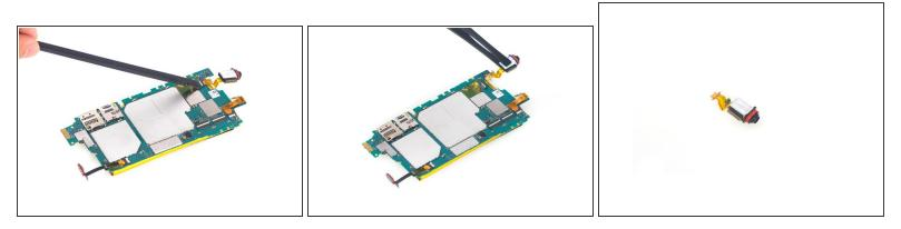
Remove audio jack flex by flipping up the white locking tab of the connector base.
