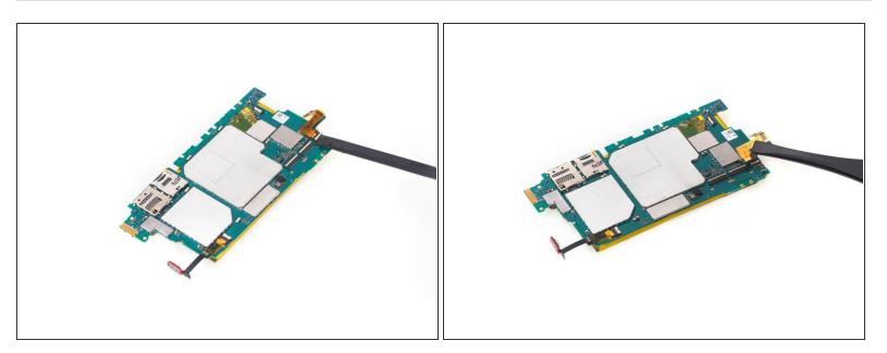
Remove flashlight flex by flipping up the white locking tab of the connector base.
