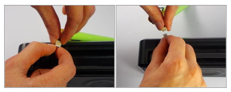
• Disconnect the old battery from the plug that is attached to the device by grabbing both ends of the plug and pulling them apart.
