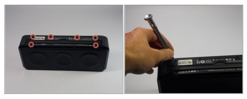
Remove all (6) 5mm Torx (Star) screws on the bottom panel of the device using the T4 screwdriver.
