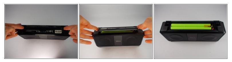
• Remove the bottom panel from the A33 by inserting both fingers in the gaps on the edge of the panel and lifting up until the bottom panel comes off of the device.
