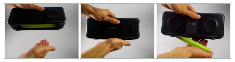
$\bigwedge$  Do not rip the wires connecting the A33 to the battery when removing the battery from the device.
