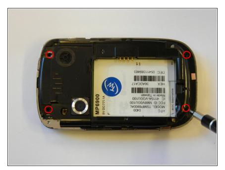
Remove the 4 torx-head screws in the corners of the phone using the T5 Torx Screwdriver.
