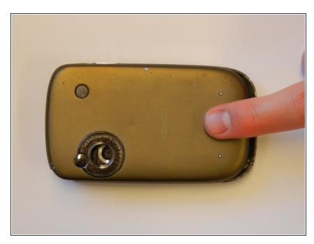
Remove the back panel by sliding it up.
