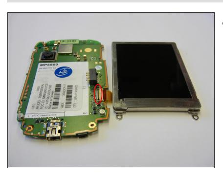
Lift the black lever next to the orange ribbon cable to remove the LCD screen.
