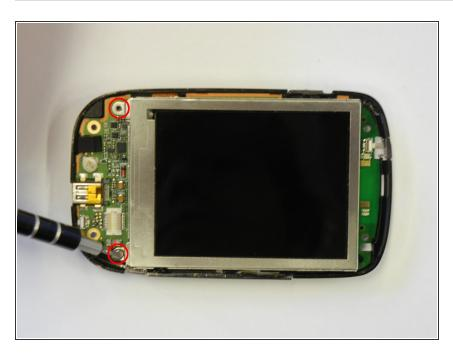
Unscrew the 2 torx-head screws at the base of the LCD screen using the T5 Torx Screwdriver.
