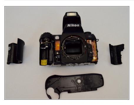
Separate the three front camera plates from the camera.
