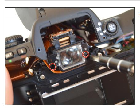
Remove the two 4.8mm screws next to the viewfinder with a PH00 Phillips screwdriver.
