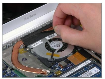
Carefully peel up the black felt tape between the heat sink and fan.
