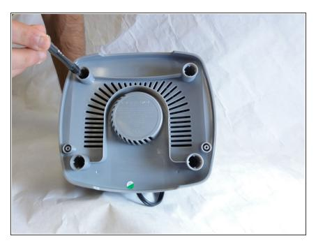
Unscrew all 4 screws that are located beneath the pads with a screwdriver and remove the plastic grey base.
