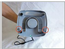
Hold the food processor upside down and remove the two screws indicated with a screwdriver.
