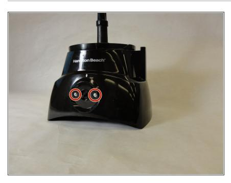
Remove the two screws behind the knob with a screwdriver.
