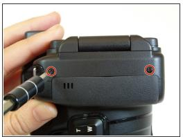
• Use a Phillips screwdriver and remove the eleven 5.556 mm screws around the outside frame of the camera.
