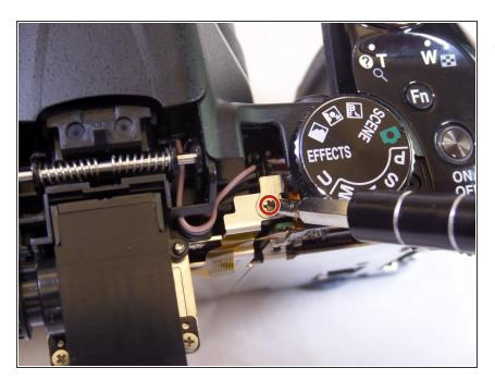
Use a Phillips screwdriver and remove the single 6.350 mm screw, left of the mode-adjustment dial.
