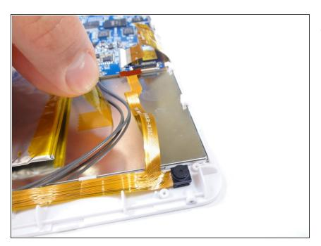
• Carefully remove the tape of the ribbon cables attached to the camera.
