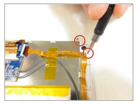
• Remove the two screws holding the internal camera in place.
