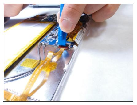
Using a plastic opening tool, lift open the tab that holds the connection between the camera and motherboard in place. The ribbon cable will become detached.
