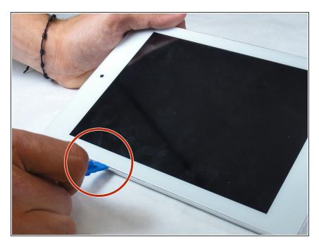
Pry the back case off using the blue <u>Plastic Opening Tools</u>. Work one along the seem until you can get your fingers under to pull it apart.
