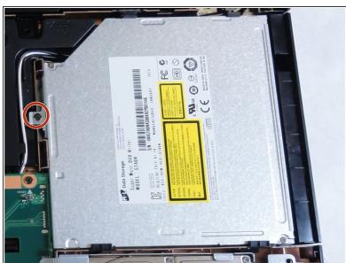
Remove the single screw that is holding the drive in place using the Phillips #1 Screwdriver.
