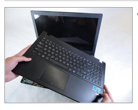
Remove the fully disconnected keyboard module from the laptop.
