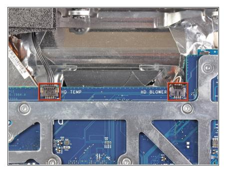
Disconnect the hard drive thermal sensor and hard drive fan cables from the logic board by pulling their connectors toward the top edge of the iMac.
