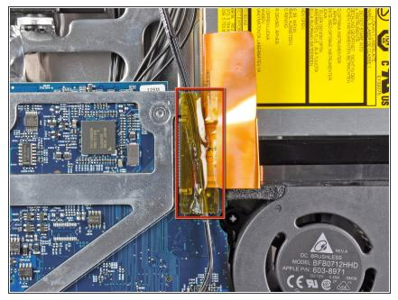
i If necessary, remove the strip of tape covering the optical drive connector.
