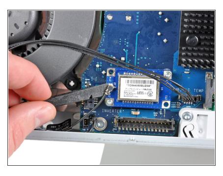
Use the flat end of a spudger to pry the single Bluetooth antenna off its socket on the Bluetooth board.
