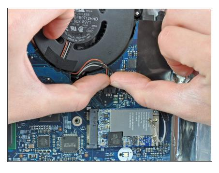
Pull the optical drive fan connector toward the top edge of the iMac to disconnect it from the logic board.
