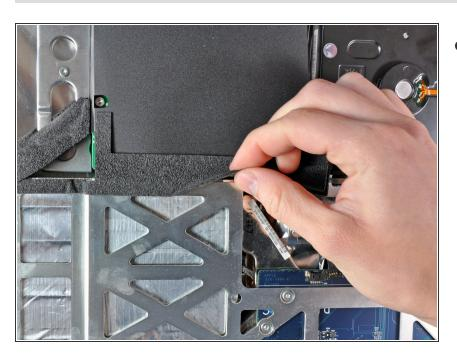
Peel the foam tape off the top edge of the heat sink framework.
