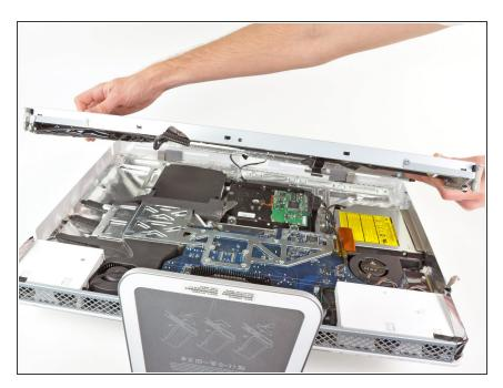
Remove the display assembly from the iMac.
