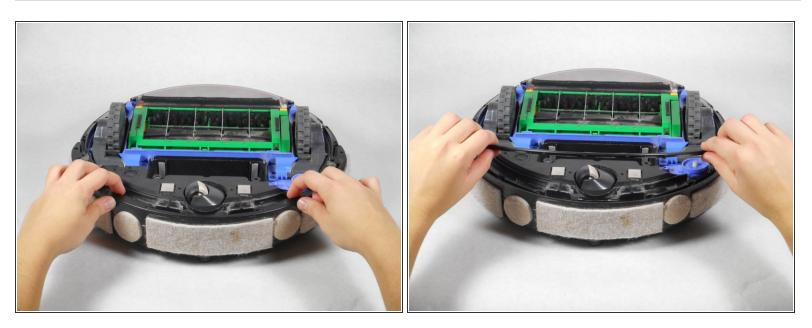
• Lift the thin top cover that holds the bumper in place.
