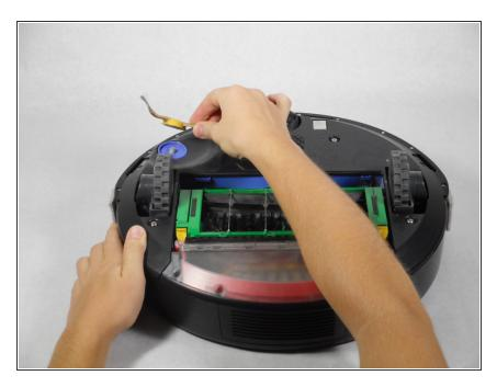
• Lift the yellow side sweeper, removing it from the device.
