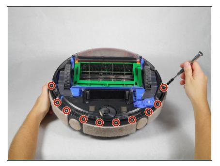
Using the Phillips #1 driver, remove the ten 10 mm screws on the bumper that run along the outer edge of the Roomba.
