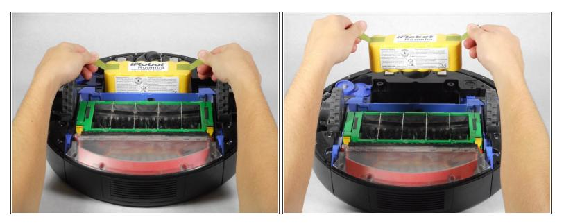
Lift up the yellow battery by pulling up the green tabs on its side.
