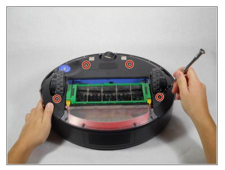
Using the Phillips #2 driver, remove the four 10 mm screws that hold the back panel in place.
