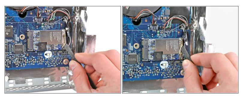
• Use the flat end of a spudger to pry both antenna connectors off their sockets on the AirPort card.
