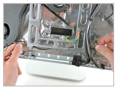
• De-route the left speaker cable from beneath the framework near the center of the iMac.
