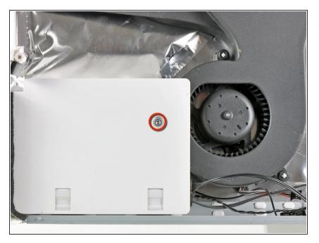
Remove the 38 mm T10 Torx screw securing the left speaker to the rear case.
