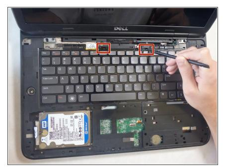
Use a spudger to release both clips that hold the keyboard in place.
