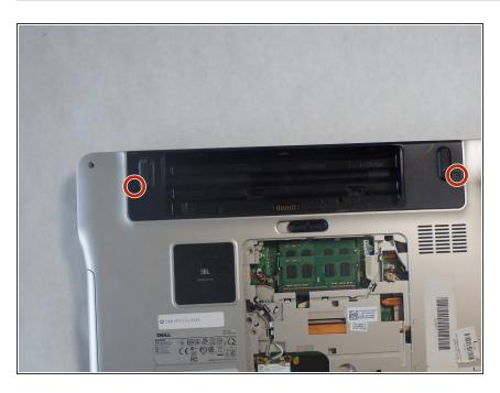
Flip the computer over and remove the two 5 mm Phillips screws on both sides of the battery terminal using a Phillips screwdriver.
