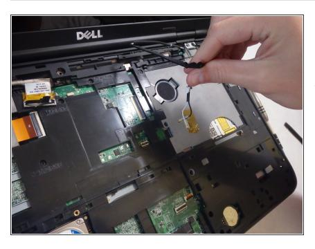
Flip the computer back over into its upright position and gently pull the wires away from their prior points of connection while making sure not to damage them.
