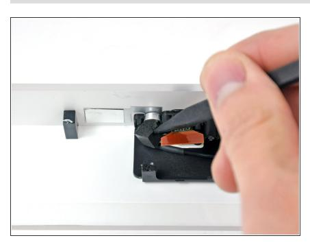
Use the tip of a spudger to remove the foam bumper covering the microphone.
