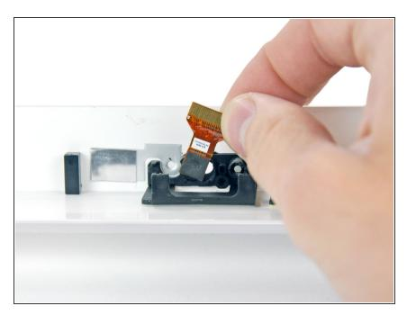
Pull the camera lens away from the camera bracket and remove it from the front bezel.
