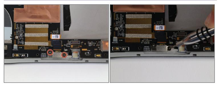
• Remove the two 4mm screws with the T5 Torx Screwdriver.
