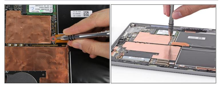
Remove the 3 mm T3 Torx screw securing the battery connector, and disconnect the battery connector.
