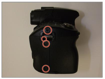
• Remove three screws from the right hand side of the case.
