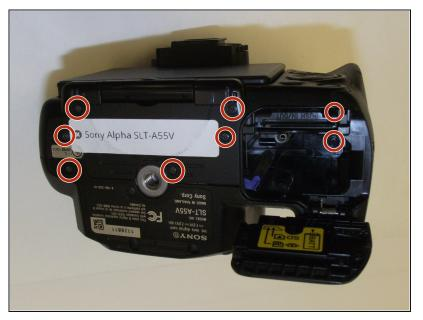
On the bottom of the camera remove seven screws indicated by the circles in the picture to the left.
