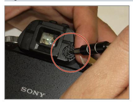
Remove the screw that attaches the focusing adjustment for the eyepiece.
