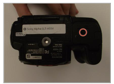
Locate the battery compartment on the bottom of the unit. Then, slide the latch down to open the cover.
