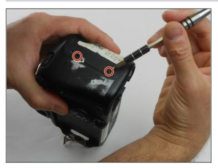
Remove two 4.8 mm Phillips #PH00 screws from the memory card side of camera using the PH00 screwdriver.
