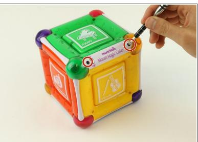
Remove two 6 mm Phillips #2 screws on either side of the On/Off Plate.
