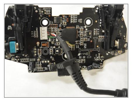
Using your new cable, solder the white connector to the logic board.
