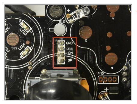
The cable connects to the logic board with a white connector. Above the right joystick, there are four solder pins labeled GND, VCC, DM, and DP.
