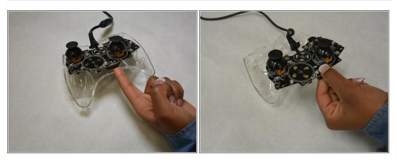
• Remove the logic board by lifting up on the logic board and pulling out.
