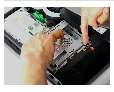
Pull up on the hard drive bay handle and push it to the left while holding back the metal tab on the bottom.
