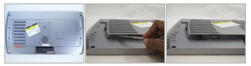
• Remove USB port cover from back plate with a metal spudger.
